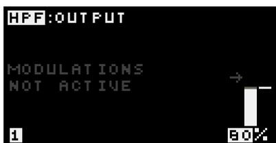
With this setup the audio from the mixer passes through a band-pass filter with fixed width and a centre frequency around 1.5kHz. Of course the frequencies of the low and high pass filters can be modulated (independently) to make the sound more interesting.
