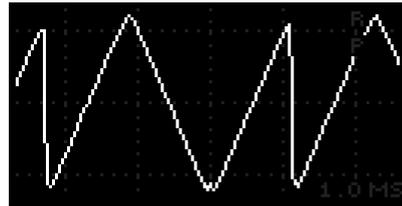
In a more complex example the waveform below shows the triangle wave output of oscillator 1 which is synced to oscillators 2 and 3. The frequency of oscillator 2 is set to 7 semitones lower than oscillator 1 whilst the frequency of oscillator 3 is set to 9 semitones lower. The triangle waveform is distorted with 2 resets during its cycle.
