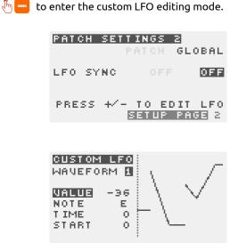
Any LFO (parameter-page local, or global) can use the 4 custom LFO waveforms just like the preset waveforms.
