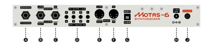
The lettering at the top of the rear panel is printed upside down so that the user can read the lettering when peering over from the top of the unit.
