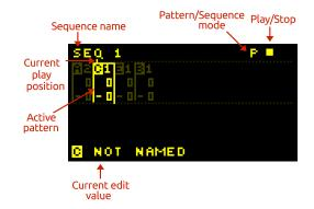
Press  $\bigcirc$   $\bigcirc$  to insert a pattern at the current point or press  $\bigcirc$   $\bigcirc$  to remove a pattern from the sequence. Use the  $\bigcirc$   $\bigcirc$  and  $\bigcirc$   $\longrightarrow$  to move between the patterns in the sequence. A pattern in the sequence is active when brighter than the other patterns.
