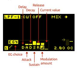
When delay time  $\frac{1}{2}$  when delay time  $\frac{1}{2}$  is the active option envelope rises after the delay phase, pressing  $b \leftarrow$  and  $b \rightarrow$  selects from the EG trigger mode options. The selected mode is shown as a small icon on the screen to the left of the delay **I** icon, from the following 8 options:
