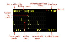
The active pattern can be selected using the  $\frac{1}{2}$  and  $\frac{1}{2}$  buttons. There are 15 to choose from **a**, **b**...**b**. Each can be re-named when they are saved.
