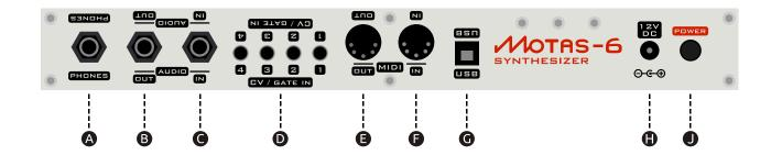
The lettering at the top of the rear panel is printed upside down so that the user can read the lettering when peering over from the top of the unit.
