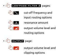
Use the 'page-lock' mode to allow rapid hands-on changes of parameter basic offsets such as sweeping filter cut-off, changing oscillator mix levels etc. without changing the active parameter page. Press the PAGE LOCK button to toggle 'page-lock' on and off. When 'locked' the LED will flash next to the PAGE LOCK button.
