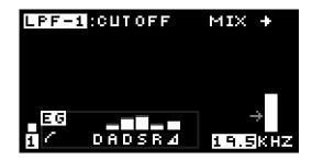
For example, the figure above shows the parameter page for the low-pass filter 1 cut-off frequency. Here there is an EG set and the basic offset (ignoring modulation) has the cut-off frequency set to 19.5 kHz.
