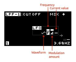
To change the LFO waveform press the  $(a) \land a$  for  $(a) \land a$  then use the rotary encoder (a), or press  $(a) \land a$  or  $(a) \lor a$ , to change the waveform. The current setting will be shown on the display. Press  $(a) \land a$  and  $(a) \lor a$  simultaneously to reset the waveform to a sine wave. See section 9.2 for a list of the available waveforms.
