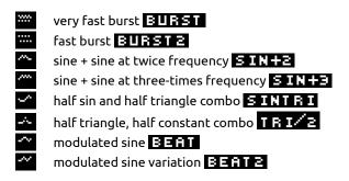
The next 17 waveforms are primarily aimed at pitch modulation of the oscillators to play tuned notes (but of course you don't have to do that!). They give the intended pitch with an LFO amount set to 12.00s
