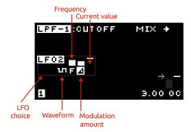
The global LFOs are useful when the same LFO modulation signal is desired applied to more than one destination, e.g. a tremolo modulation (volume modulation) at the same frequency as vibrato (pitch modulation). Note that although the LFOx are global, the level applied to each destination is independent.
