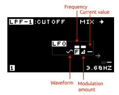
To change the LFO waveform press the for LFD then use the rotary encoder (0, 0), or press (0, 0) or (0, 0) (0, 0) (0, 0) or (0, 0) (0, 0) or the display. Press (0, 0) and (0, 0) simultaneously to reset the waveform to a sine wave. See section 9.2 for a list of the available waveforms.
