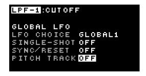
Use [BUTTON-UP] and [BUTTON-DOWN] to choose which LFO option to edit and the [ROTARY ENCODER] to change the values. There are 4 options:
