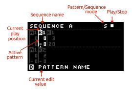
Press to insert a pattern at the current point or press to remove a pattern from the sequence. Use the and to move between the patterns in the sequence. A pattern in the sequence is active when brighter than the other patterns.
