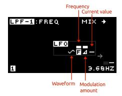
To change the LFO waveform press the for then use the rotary encoder O, or press of or to change the waveform. The current setting will be shown on the display. Press of and to simultaneously to reset the waveform to a sine wave. See section 9.2 for a list of the available waveforms.
