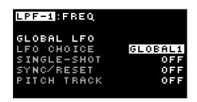
Use  $\frac{1}{2}$  and  $\frac{1}{2}$  to choose which LFO option to edit and the rotary encoder  $\stackrel{\checkmark}{O}$  to change the values. There are 4 options:
