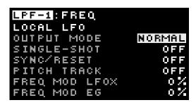
Use the [BUTTON-UP] and [BUTTON-DOWN] buttons to choose which LFO option to edit and the [ROTARY ENCODER] to change the values. There are 6 options:
