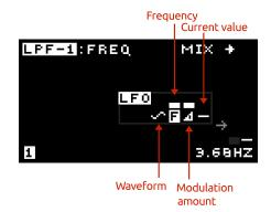
To change the LFO waveform press the [BUTTON-LFO WAV-FORM] for local LFO then use the [ROTARY ENCODER], or press [BUTTON-UP] or [BUTTON-DOWN], to change the waveform. The current setting will be shown on the display. Press [BUTTON-UP] and [BUTTON-DOWN] simultaneously to reset the waveform to a sine wave. See section 9.2 for a list of the available waveforms.
