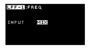
In the screenshot example shown above the option for the LPF-1 cut-off frequency page is the source of the audio input to the filter. In this case this input is set to 'mix'.
