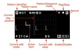
The active pattern can be selected using the [BUTTON-LFO X WAVEFORM/INCREASE] and [BUTTON-LFO X FREQUENCY/DECREASE] buttons. There are 15 to choose from A, B ...O. Each can be re-named when they are saved.
