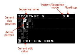
Press [BUTTON-LFO X WAVEFORM / INCREASE] to insert a pattern at the current point or press [BUTTON-LFO X FREQUENCY / DE-CREASE] to remove a pattern from the sequence. Use the [BUTTON-LEFT] and [BUTTON-RIGHT] to move between the patterns in the sequence. A pattern in the sequence is active when brighter than the other patterns.
