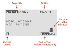
At the far right of the main parameter display a horizontal bar shows the current level of the destination signal in real time. The current value is the sum of the basic offset for the page with all the modulation signals (see chapter 9 for explanation of the modulation options).
