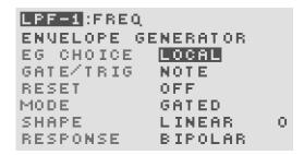
Use [BUTTON-UP] and [BUTTON-DOWN] to choose which EG option to edit and the [ROTARY ENCODER] to change the values. There are 6 options.
