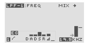
For example, the figure above shows the parameter page for the low-pass filter 1 cut-off frequency.
