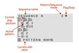
Press b c to insert a pattern at the current point or press b  $\fbox{c}$  to remove a pattern from the sequence. Use the b  $\Huge{c}$  and b  $\Huge{c}$  to move between the patterns in the sequence. A pattern in the sequence is active when brighter than the other patterns.
