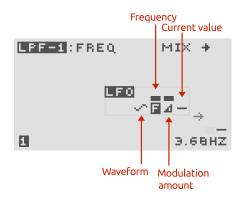
To change the LFO waveform press (0, or press, 1) for **LFD** then use the rotary encoder (0, or press, 1) or (0, 1), to change the waveform. The current setting will be shown on the display. Press (0, 1) and (0, 1) simultaneously to reset the waveform to a sine wave. See section 9.2 for a list of the available waveforms.
