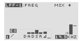
For example, the figure above shows the parameter page for the low-pass filter 1 cut-off frequency.
