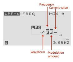
To change the LFO waveform press [BUTTON-LFO WAVFORM] for local LFO then use the [ROTARY ENCODER], or press [BUTTON-UP] or [BUTTON-DOWN], to change the waveform. The current setting will be shown on the display. Press [BUTTON-UP] and [BUTTON-DOWN] simultaneously to reset the waveform to a sine wave. See section 9.2 for a list of the available waveforms.
