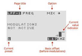
At the far right of the main parameter display a horizontal bar shows the current level of the destination signal in real time. The current value is the sum of the basic offset for the page with all the modulation signals (see chapter 9 for explanation of the modulation options).
