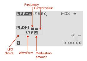
[TIP] The global LFOs are useful when the same LFO modulation signal is desired applied to more than one destination, e.g. a tremolo modulation (volume modulation) at the same frequency as vibrato (pitch modulation). Note that although the LFOx are global, the level applied to each destination is independent.
