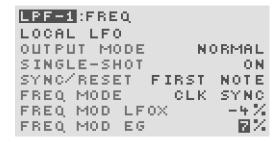
Use the [BUTTON-UP] and [BUTTON-DOWN] buttons to choose which LFO option to edit and the [ROTARY ENCODER] to change the values. There are 6 options:
