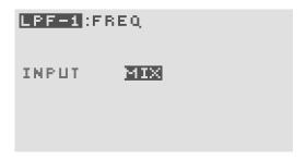
In the screenshot example shown above the option for the LPF-1 cut-off frequency page is the source of the audio input to the filter. In this case this input is set to 'mix'.
