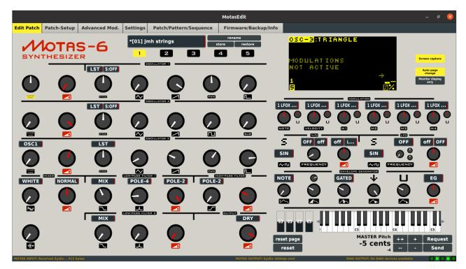
To receive live screenshots from Motas-6 select the 'Screen capture' button. This causes the software to request screen data via SysEx commands and then Motas-6 sends the screen data. Due to the large amounts of data in this process the operation of Motas-6 may then be rather sluggish, especially if the setting SYSEX EX OUT DELAY on Motas-6 is increased. However, this does not affect the sound from Motas-6 only the user interface.
