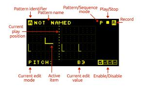
The active pattern can be selected using the  $\frac{1}{2}$  and  $\frac{1}{2}$  buttons. There are 15 to choose from **(a)**, **(b)**. Each can be re-named when they are saved.
