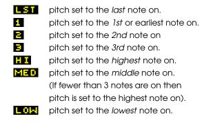
Additionally, the behaviour of the pitch tracking on note-off events is determined by a global patch setting **TRACK NOTE-OFF** for all oscillators. See section 18.1 for more details. In some modes, with this feature turned on, the pitch will change to track the remaining notes pressed as others are released.
