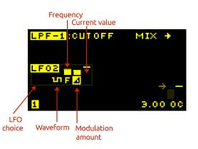
The global LFOs are useful when the same LFO modulation signal is desired applied to more than one destination, e.g. a tremolo modulation (volume modulation) at the same frequency as vibrato (pitch modulation). Note that although the LFOx are global, the level applied to each destination is independent.
