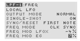
Use the [BUTTON-UP] and [BUTTON-DOWN] buttons to choose which LFO option to edit and the [ROTARY ENCODER] to change the values. There are 6 options:
