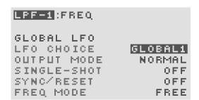
Use [BUTTON-UP] and [BUTTON-DOWN] to choose which LFO option to edit and the [ROTARY ENCODER] to change the values. There are 4 options:
